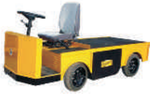
4 Wheeler Platform Truck Capacity : 2000 / 3000 Kgs
