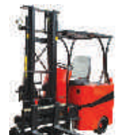
Articulated Fork Lift Capacity : 2000 Kgs Lift : 10 Meters
