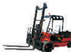
Battery Operated Fork Lift Capacity : 4000 / 5000 Kgs
