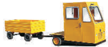
Tow Truck with Trolley Capacity : 1000/3000/5000 Kgs
