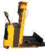
Dia Loading Stacker Capacity : 2000 Kgs
